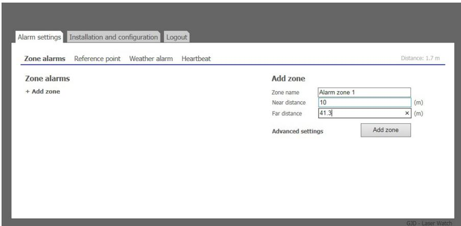
Steps 6 to 9 covers advanced settings. These settings are not necessary, but can be used to adapt the zones for special purposes. We recommend to thoroughly verify the function of the alarm zone if these settings are changed.
