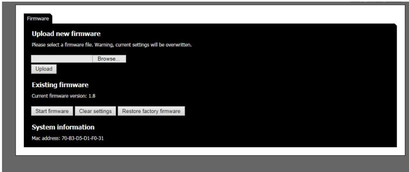
4. To restore factory settings, press Clear settings button. Press Start firmware to start the Laser-Watch firmware again.
