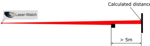
If it is less than 5 meters between the objects the sensor cluster the objects and use weighted averaging to calculate a virtual object position. If each object gets 50% of the laser beam the calculated distance will be in the middle between the objects. If the first object gets 75% and the other 25% the calculated distance will move closer to the first object.
