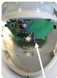
Fig.1 D-TECT IR emitter
